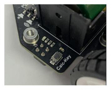
3. If all the line-tracking sensor indicators are turned on in the black area and turned off in the white area, the calibration is completed.
