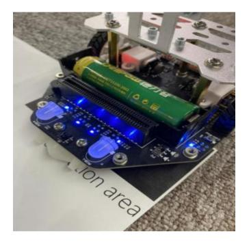
2. Press "Calc-key" for about 1 second, the 2 front large LEDs will flash in green. Upon release of the key, the calibration is completed.
