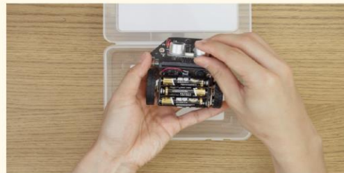
4. Install ultrasonic sensor
